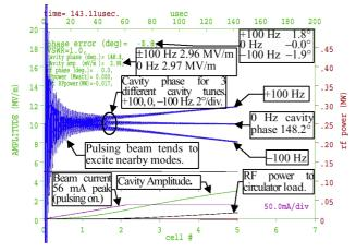
**Figure 1:** Example of phase response of superconducting cavity to 36 mA beam pulse when cavity is tuned 100 Hz high, correctly, and low 100 Hz. The phase error at 143  $\mu$ second into pulse is +1.8°, 0°, and -1.9°. Note that there is some ringing in the cavity that damps in about 60  $\mu$ s, sufficient to see the effect of the cavity tune on the phase.
