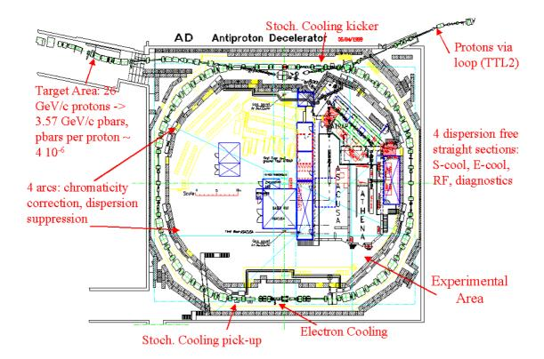
machine could be built with an investment of only 8 MCHF, necessary mainly for the upgrade and refurbishing of: vacuum, power supplies, electron cooling, rf, diagnostics, controls, and experimental areas. Compared to the scheme used until 1996 which needed four machines (the AC, AA, PS and LEAR) to provide lowenergy antiproton beams, the AD has brought considerable savings in operational cost (e.g. power consumption of only 0.5 instead of 8 MW) and manpower.
