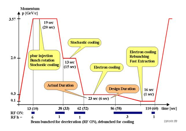
Figure 2: AD Deceleration Cycle
