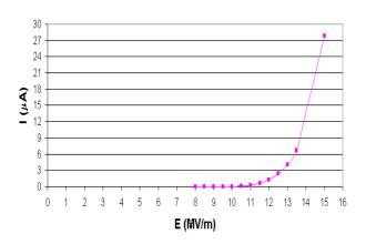
Figure 2: Field emission from a 1 µm finish stainless steel electrode
