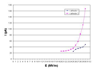
Figure 4: Field emission from two different 9 µm finish stainless steel electrodes treated by PSII/PVD
