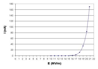
Figure 3: Field emission from a 1 µm finish Ti4V6Al electrode
