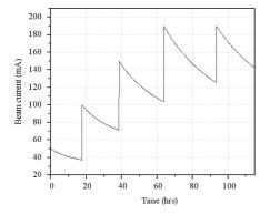
Figure 1. Beam current intensity possible scenario, during the conditioning period in the VLHC, Stage 1, increasing the current from 50mA to 190mA (nominal), in four steps.
