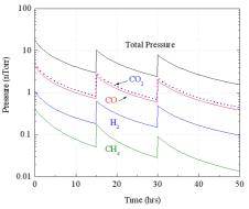
Figure 7. CO scattering equivalent partial pressures and total pressure in the possible conditioning scenario, Stage2.
