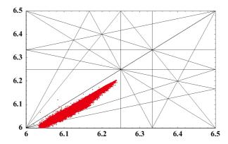
Figure 4: An example of  $(Q_x, Q_y) = (6.23, 6.2)$  working point. Tune spread (red) of a 2MW beam due to the combined effect of space-charge and  $\Delta p/p = 0.7\%$ .
