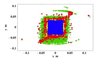
Figure 1: Blow-up of beam profile due to skew-quadrupole sum resonance in the presence of space charge: blue color (in the middle) - no space charge, no errors; yellow color - space charge, no errors; red color - space charge, expected errors and quadrupole tilt (0.2 mrad); green color - space charge, expected errors and quadrupole tilt (1 mrad).
