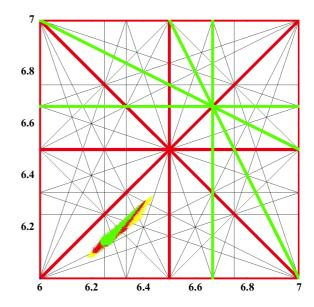
Figure 2: Working point  $(Q_x,Q_y)=(6.4,6.3)$  with a tune footprint for a 2MW beam: green color represents tune spread due to space charge alone; red color also includes momentum spread of 0.7%; yellow color shows combined effect of space charge and  $\Delta p/p=1\%$ .
