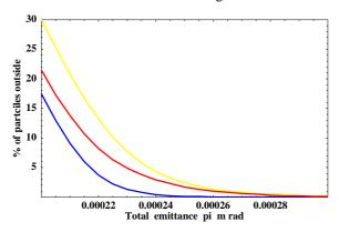
Figure 3: Beam halo due to expected magnet errors for  $(Q_x,Q_y)=(6.4,6.3)$ : blue color shows halo due space charge alone; red color corresponds to the case of both systematic and random magnet field errors at a few units at  $10^{-4}$  level, chromatic sextupoles and quadrupole fringe fields; yellow color shows an additional effect of x,y misalingments of 0.5 mm and magnet tilt of 1 mrad.
