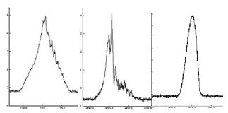
Figure 2: Instability perturbation on profiles of bunches with full width 250 ns (left) and 100 ns (middle). Right: Upon heating the ferrite to  $130^{\circ}$ C (see Sec. 4), the profile of the 100 ns bunch is no longer distorted.
