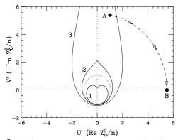
Figure 3: An intense space-charge beam may have impedance at A outside the Keil-Schnell circle (dots) but is stable inside the stability curve 3 for Gaussian distribution. Ferrite inserts compensating the space charge completely will lead to a resistive impedance roughly at B and therefore introducing instability.
