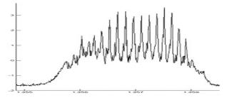
Figure 1: Longitudinal microwave-like instability recorded by wall-gap monitor of a coasting beam driven at 72.7 MHz.
