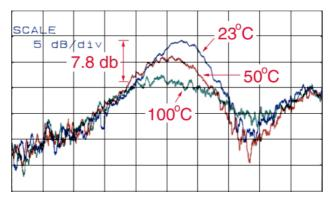
Figure 4: (color) As the ferrite cores are heated from room temperature to  $100^{\circ}$ C, the loss has reduced by almost 6 times. Abscissa: center 75.0 MHz, span 149.4 MHz. Ordinate: 5 db/div.
