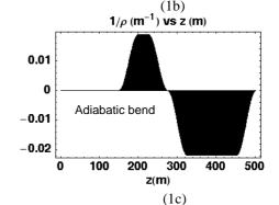
Figure 1. Inverse instantaneous radius of curvature (m<sup>-1</sup>) as a function axial distance (m) for (a) an abrupt bend, (b) a matched bend, and (c) an adiabatic bend, using
