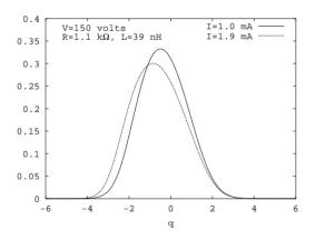
Figure 2: Equilibrium distributions in the absence of IBS (Haissinski solutions) for I=1.0 and 1.9 mA;  $q=z/\sigma_{s0}$  is the scaled longitudinal distance,  $\sigma_{s0}$  the natural bunch length in the zero-current limit.
