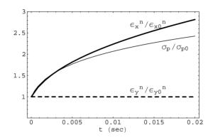
Figure 4: Evolution of (normalized) rms emittances (in m) and relative momentum spread. E = 25 MeV.
