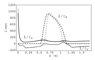
Figure 3: Local IBS growth rates along the lattice. Thick lines refer to calculation done according to Bjorken-Mtingwa; thin lines are calculated according to Piwinski. The vertical growth rate  $1/\tau_y$  is magnified by a factor 100.
