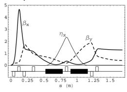
Figure 1: Lattice functions;  $\beta$ -functions are in m,  $\eta_x$  is in units of 10 cm.
