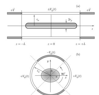
Figure 1: (a) Side view and (b) end view of Paul Trap Simulator Experiment (PTSX).
