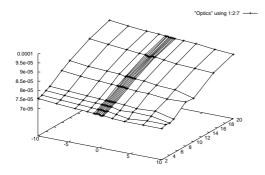
Figure 2: Emittance growth from numerical simulation for a single bend: R = 2m, L = 1m, q = 1nC, E = $40.7 \text{MeV}, \varepsilon_{\text{normalized}} = 70 \cdot 10^{-6} \text{m}$
