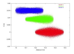
Figure 2: X - Z distribution of three beam bunches near the end of halo channel.
