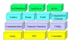
Figure 1: A schematic plot of the multi-layer structure for beam dynamics system simulations.
