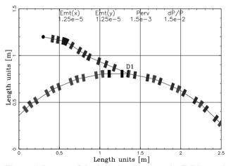
Figure 1: Layout of the injection line into the E-Ring and several sectors of the E-Ring lattice. The blackened circle denotes the input point into the injection system.
