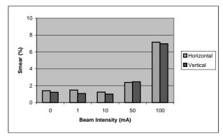
Figure 5: Horizontal and vertical smear values of E-Ring lattice vs. beam current with adjusted quadrupole settings.
