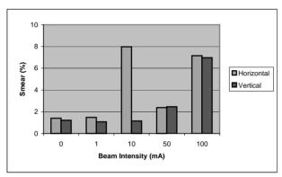
Figure 4: Horizontal and vertical smear values of E-Ring lattice vs. beam current with fixed lattice quadrupole settings.
