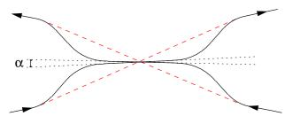
Figure 3: Trajectories through the IR with a crossing angle  $\alpha$ . The dashed (red) lines show how the crossing angle increases without the DX magnets.
