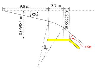
Figure 4: Aperture limit of trajectory through DX magnet. The warm beam pipe extends about 25.6 cm beyond the end of the DX magnet before bending towards the D0 magnet.[2]
