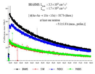
Figure 7. Luminosities at all four experiments measured by the Zero-degree calorimeters.
