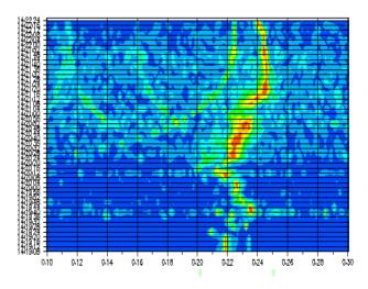
Figure 4. Horizontal betatron tunes along the RHIC acceleration.
