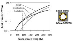
Figure 2: Heat Transfer from beam-screen to cold-bore.
