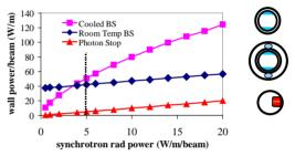
Figure 5: Wall power density vs. SR load for different solutions(cold BS, warm BS/shield and PS).
