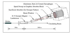
Figure 3: Schematic layout of beam abort channel.
