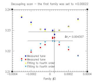
Figure 4: Coupling correction for the Blue ring in 2001.
