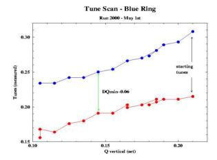
Figure 2. First tune scan in RHIC to measure  $\Delta$ Qmin in the Blue Ring.
