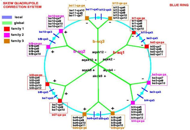
Figure 1: Schematic view of the skew quadrupole correction system in the RHIC Blue ring.
