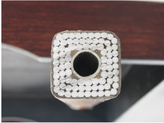
Figure 3: Water-cooled Stranded Conductor Cross-section.
