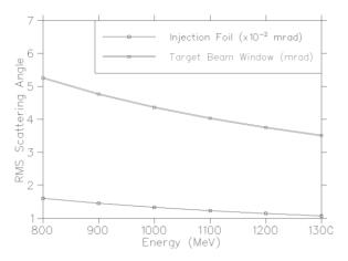
**Figure 4:** RMS multiple scattering angles as a function of energy for proton beam window in RTBT which is 4 mm thick made of inconel and injection carbon foil  $300\mu$ g/cm<sup>2</sup>.
