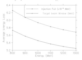
**Figure 3:** Average energy loss as a function of energy for proton beam window in RTBT which is 4 mm thick made of inconel and injection carbon foil  $300 \ \mu g/cm^2$ .
