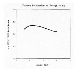
Figure 5: Neutron yield per MW of beam power for a lead target.
