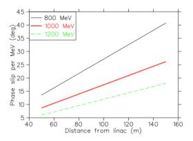
Figure 1: Phase slip per MeV as a function of distance between the last linac cavity and energy corrector cavity.
