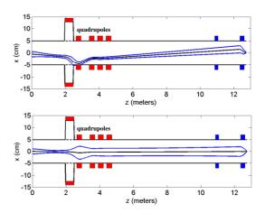
Figure 6: Beam envelopes during the kicker switch phase and at steady state. The kicker exit is at z=0.
