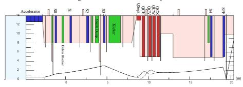
Figure 2: Transport simulation showing DARHT-II beam envelope from accelerator exit to x-ray converter target.
