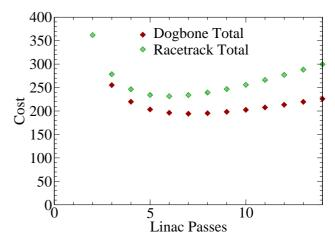
Figure 2: Total system cost as a function of the number of passes through a given linac.
