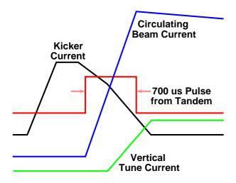
Figure 2: Typical Timing at Booster Injection.
