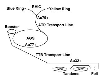
Figure 1: Acceleration of Gold Ions for RHIC.
