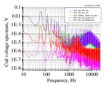
Figure 4: Coil voltage spectra.
