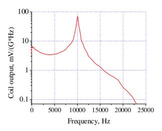
Figure 2: Sensitivity of the measurement coil.
