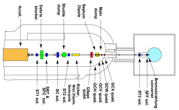
Figure 1: Layout of the transport elements.
