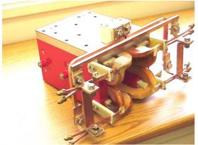
Figure 2: Picture of a Collins Quadrupole.
