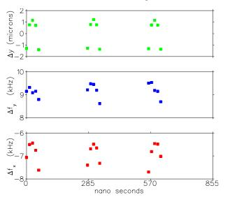
Figure 1: Tune shift in one beam due to long range interaction with the opposing beam. There are 9, 5-bunch trains with 7.5mA/bunch in each beam. Bunch spacing within each train is 14ns.  $f_{rev} = 390.1$ kHz. The difference in the vertical orbits at the IP for the two beams is shown above.
