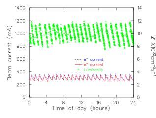
Figure 5: Beam current and luminosity during a 24 hour period. Total luminosity for the day is  $73pb^{-1}$
