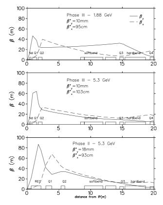
Figure 7: Exisiting IR with 1.5m permanent magnet quad at bottom. Superconducting IR quad layout and optical functions for 5.3GeV and 1.88Gev are above.
