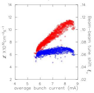
Figure 3: Average beam-beam tune shift  $\xi_v$  and luminosity versus bunch current with nine, 4-bunch trains/beam.
