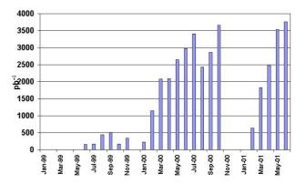
Figure 3: Monthly integrated luminosity delivered by PEP-II to BaBar.
