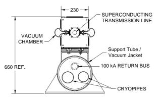
Fig. 1: "Transmission line" magnet cross-section.
