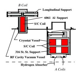
Fig. 4: Muon cooling solenoids
