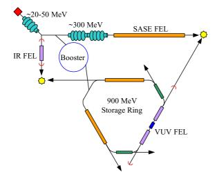
Figure 1. Schematic layout for storage ring based 4GLS. Possible combined pump-probe experiments have been highlighted.
