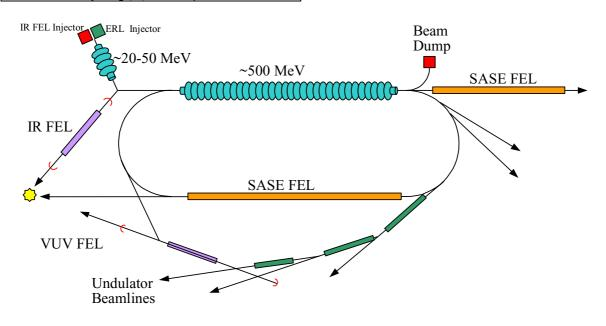
Figure 2. Schematic layout for energy recovery linac based 4GLS.
