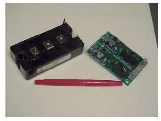
Figure 4: IGBT PM150DSA120 and IGBT Driver.
