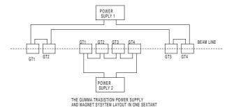
Figure 1: γT P.S. and Magnet system Layout Diagram
