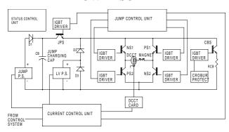
Figure 3. GT Power Supply Diagram
