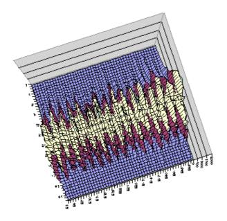
Figure 2: Mountain-range plot of the profile of a single bunch for 50 turns at injection. The detector channels are plotted on the vertical axis and the turns are on the horizontal axis.
