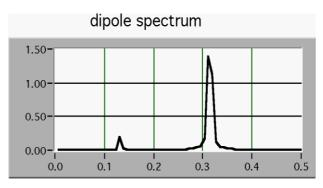
Figure 4: The power spectrum of the beam centroids on 128 consecutive turns. The line at 0.13 is the horizontal tune and 0.32 is the vertical tune.
