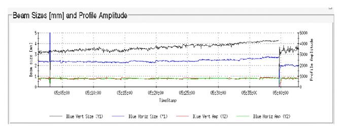
Figure 6: Vertical (top trace) and horizontal (middle trace) beam widths of a single bunch plotted at 4-second intervals for 40 minutes. At 05:40 the bunch was dumped and a new one injected.
