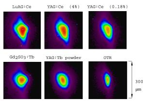
*Figure 3*: Beam images taken consequently with the six different diagnostics under the stable experimental conditions (the charge Q  $\sim$  500 pC).
