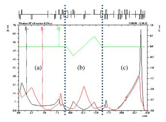
*Figure 1*: Evolution of the electron beam  $\beta$ -functions and a dispersion function along (a) post linac focusing channel; (b) dispersion section; (c) beam line 1 focusing optics.
