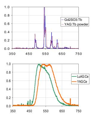
*Figure 5*: Spectral profiles of Tb doped and Ce scintillators emission respectively, under the electron beam excitation. Small dip at 550 nm in the YAG:Ce emission profile was very distinct and repeatable.
