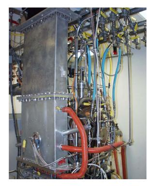
Figure 4: rf test cavity assembly.
