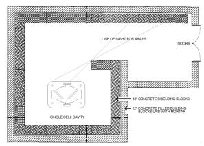
Figure 2: Test bunker top view.
