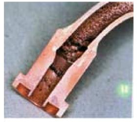
Figure 5: Original step at the welding position becomes too smooth. Water flows from upper to bottom.
