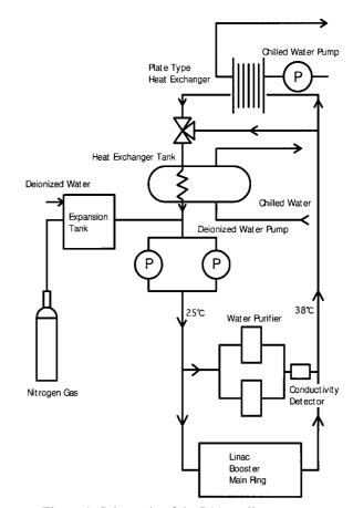
Figure 1: Schematic of the P11 cooling system.
