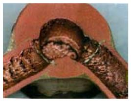
Figure 6: Evidence of the erosion by cavitation. Water flows from right to left.
