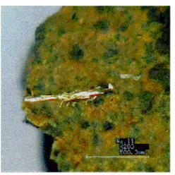
Figure 7: Inner surface of the rubber tube for the field monitor bending magnet.
