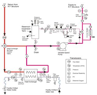
Figure 2. Flow diagram of the DTL and CCL water cooling systems.
