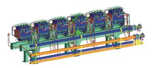
(b) Figure 1. (a) DTL tank and (b) CCL half module.
