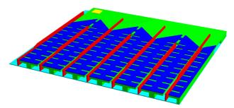
Figure 1: A part of the meander structure model: notched metal meander strip (dark-blue) on dielectric supports (green), metal separators (red) are connected to the ground plate (light-blue, below).
