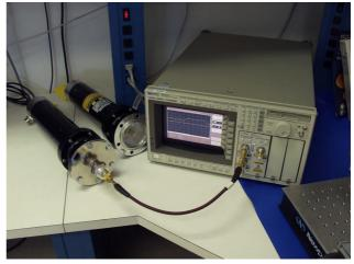
Figure 6: Bird Electronics 8775 load is being tested with the time-domain reflectometer.
