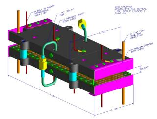
Figure 3: Assembled current plates of the MEBT chopper.
