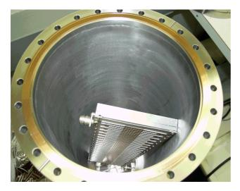
Figure 5: The prototype current structure in the vacuum test chamber.
