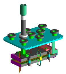
Figure 4: Chopper assembly mounted on the vacuum box lid (courtesy of Daryl Oshatz, LBNL).
