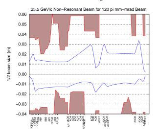
Figure 1: 1/2 horizontal and vertical beam sizes for transport to the muon collider target.
