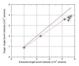
Figure 4: Target beam intensity vs extracted beam intensity. The red line corresponds to a 100 % transmission, to guide the eye.
