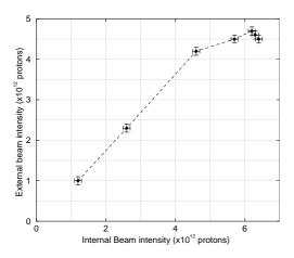
Figure 5: extracted beam intensity versus internal intensity
