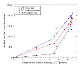
Figure 4: Beam losses versus intensity (loss monitors have roughly equal response to a given amount of lost beam)
