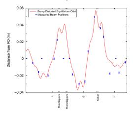
Figure 2: Measured orbit points and the predicted orbit around the kicker and septa locations.
