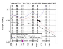
Figure 3: Central trajectories of kicked and unkicked beam. The location of the thin and thick septa are marked on the figure. The location of the vertical sextupole at F7 is marked in color. The solid black line is the unkicked central beam orbit. The red dotted line is the displaced orbit due to the G10 kicker. The dashed blue line is the final trajectory including the thin and thick septa bends.
