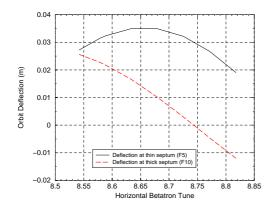
Figure 1: Central trajectory displacement as a function of horizontal tune at the location of the thin and thick septa, for a 1.8 mrad kick at 24 GeV
