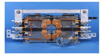
Figure 2: 3.2-cm bore quadrupole and 3- cm BPM.
