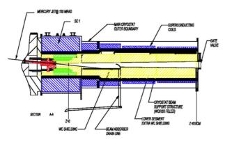
Figure 2: Sketch of the target and capture system based on a mercury jet inside a 20-T solenoid magnet.
