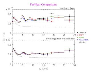
Figure 2: "Far over Near Ratio", F/N, calculated with Geant/FLUKA, MARS, BMPT, and Malensek models, along with a naive calculation assuming just the pion life-time dominates this calculation for the PH2LE beam.
