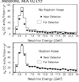
Figure 1: Neutrino energy spectra in the far and the near  $(\times 10^{-6})$  MINOS detectors with and without the Hadronic Hose for the NuMI low-energy beam (PH2LE).
