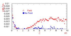
Figure 5: Energy deposited in the Hadronic Hose wire from unreacted protons, for the hose current on and off, as a function of length along the hose. The first 2 m of hose wire is not pulsed and absorbs 'head-on' protons.
