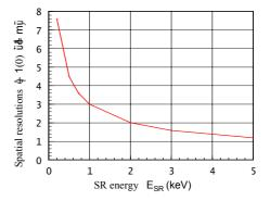
Figure 2: Spatial resolution of equation (10) as a function of the SR energy.
