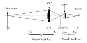
Figure 1: Layout of x-ray imaging optics
