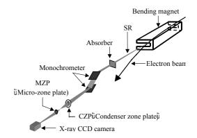
Figure 3: Schematic view of the beam size monitoring system for the Super-SOR ring.
