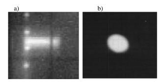
Figure 5: Beam image a) at the entrance of LM, b) at the exit window.
