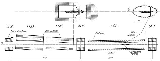
Figure 4: Layout of the extracted beam position in the fifth strait section (sizes in mm).
