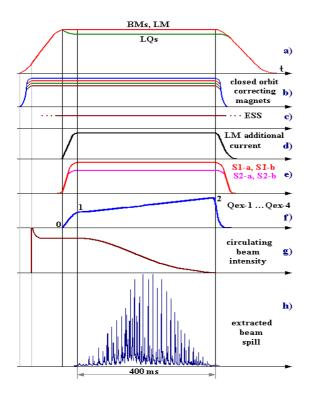
Figure 2:Timing diagram of the extraction processes.
