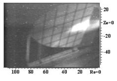
Figure 3: Image of the beam on the fluorescent screen.
