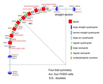
Figure 1: Schematic layout showing dipole, quadrupole, sextupole and correctors of one lattice super-period.
