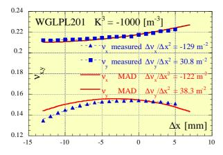
Figure 5: Comparison between measured and simulated tunes versus horizontal closed orbit bump.
