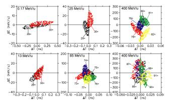
Figure 2: Longitudinal phase spaces at several stages of the linac. Upper plots: single charge stripping station at 25 MeV/u. Lower: two charge stripping stations at 13 and 85 MeV/u.
