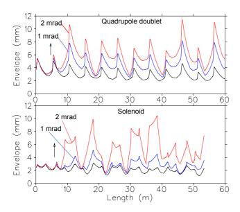
Figure 4: Beam envelopes resulting from rotational misalignment of the focusing elements for values of 0, 1 and 2 mrad. The arrows indicate the locations of misaligned elements.
