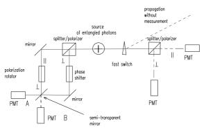
Figure 1 Experimental set-up with interference pattern to disappear at the left if the polarization measured at the right.
