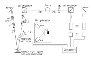
Figure 2 Proposed experimental setup. Two polarimeters I, in orientation a, and II, in orientation b, split the first photon to produce polarized electrons (at the left part) and to direct the second one to two photomultipliers (at the right side). Each polarimeter is rotatable around the axis of the beam.
