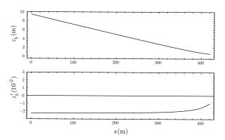
Figure 1: Longitudinal drift compression of a heavy ion fusion beam.
