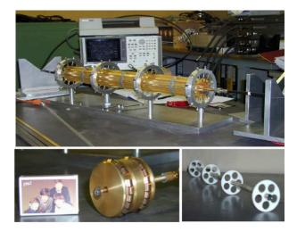
Figure 2: Q-factor measurements set-up.
