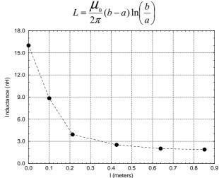
Figure 4: Inductance vs. *l* (corresponding to taper angle changes), the results displayed by dots are simulated using the ABCI (2D) code.
