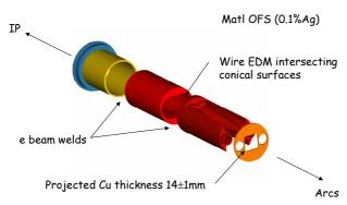
Figure 3: The TAN beam tube transition where two small beam tubes merge to a single large one at the IP.
