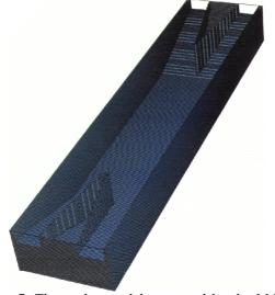
Figure 7: The wedge model generated by the MAFIA used for studying the trapped modes. Dimensions for the
