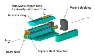
Figure 1: Exploded view of the TAN vacuum chamber A horizontal mid plane section of the TAN design is shown in Figure 2 to illustrate more details of the
